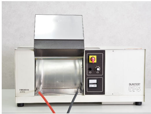
Figure 3. Heraeus Sun test CPS Accelerated Light aging chamber
