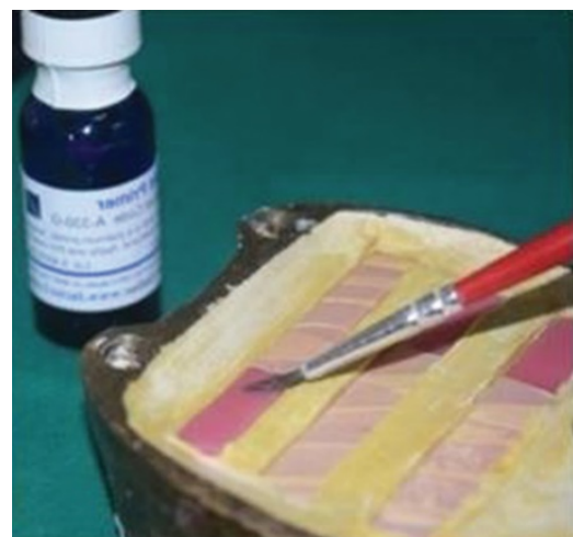
Figure 2. Adhesive primer painted on acrylic resin samples prior to addition of maxillofacial silicone
